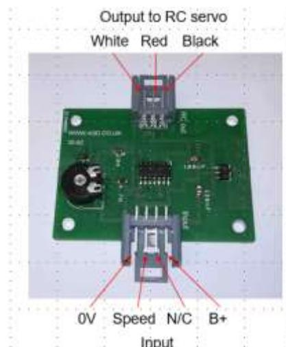
The SCC-001 can also work with other controllers by feeding a speed related positive voltage into the speed terminal, and then adjusting the pot as required.
