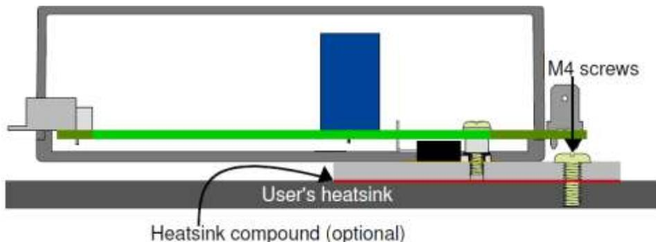
The flat aluminium plate should be bolted onto the metalwork of the machine to act as an additional heatsink, as shown above.
