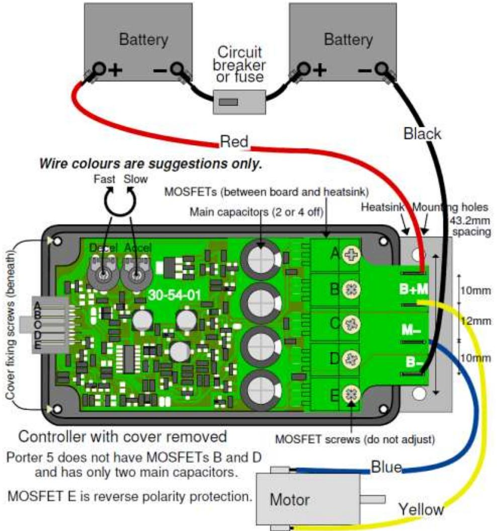
Figure 1: Porter Wiring
