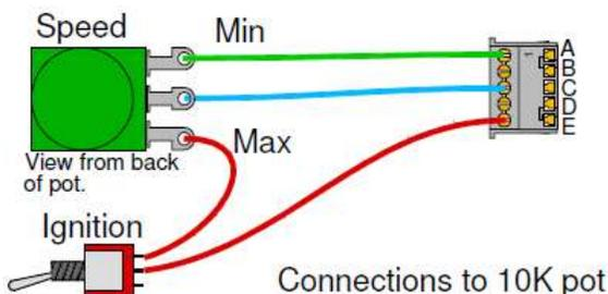
ones or external] to get an input voltage between 1V & 4V to avoid dead areas at the top and bottom of the pot travel. The ideal value of the resistors is 1/3 of the pot value.
