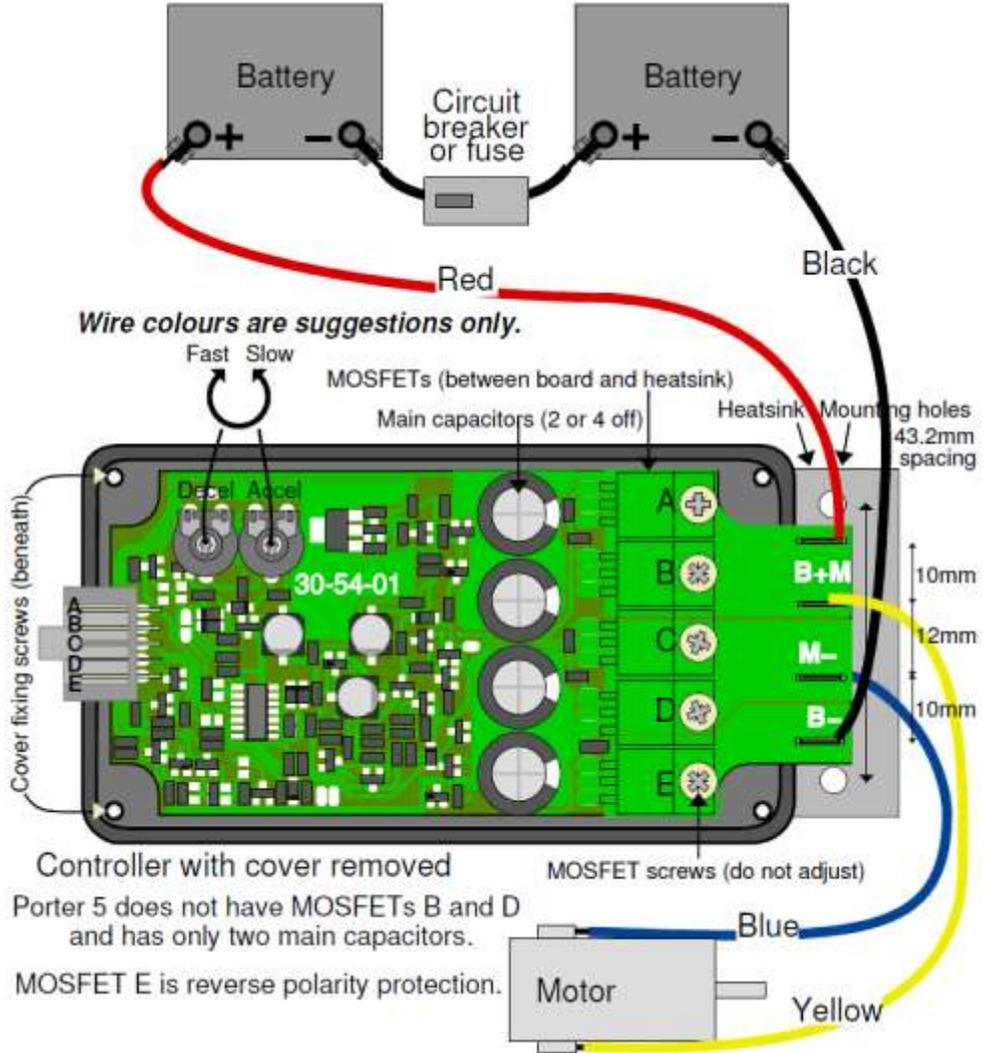
Figure 1: Porter Wiring
