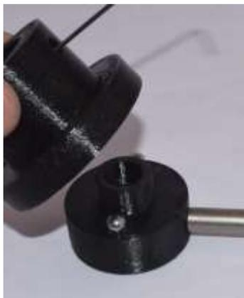
5. Carefully pick up all three parts and tighten the handle retaining screw.
