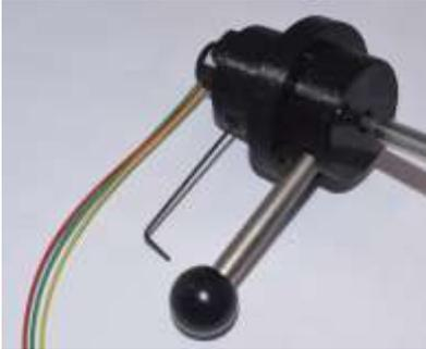
3. Place the JSK-120 handle side down and lift off the collar / drum / sensor assembly. Take care to retain the ball bearing, spring and serrated washer.
