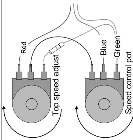
Too high a setting and there will be a 'flat' spot at maximum speed where the control has no effect. This will also confuse the special 'power down' circuitry so you will get a bumpy ride if you switch off at speed.
