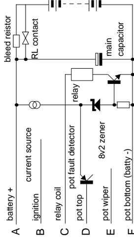
circuit, which removes all internal power. The zener also feeds a transistor which turns on the power relay as soon as the internal 9v rail establishes. The relay coil is fed from the main capacitor (via pin C of the input connector, which must be connected to pin A) which has already charged up through the bleed resistor. The relay shorts out the bleed resistor applying full power to the circuit.
