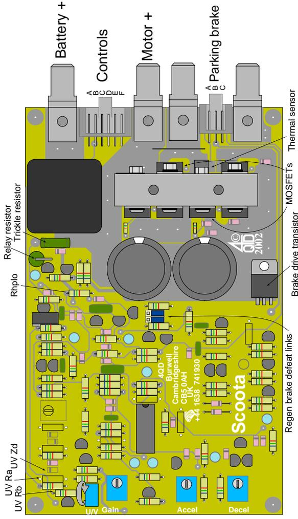
The diagram above shows the standard Sco-120 which has six 9.5mm tabs fitted: singles for the battery and doubles (for one or two motors) as shown above and in the top diagrams to the right.
