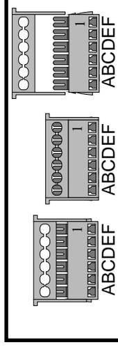
With the connector open, push the wires into the holes in the cable grip from the front which is as illustrated. The back has circular holes, not a slot.
