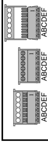
With the connector open, push the wires into the holes in the cable grip from the front which is as illustrated. The back has circular holes, not a slot.
