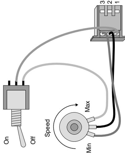
Beware of opening the switch when the motor is running: the motor will quite quickly be braked to a halt with possible high stress on the mechanics. The Mk 7 2QD has regen current limit, so it will not be damaged by this.
