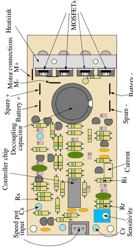
The diagram shows the 70 amp model. The 35 amp version is the same, but with only 2 MOSFETs.
