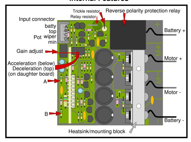
Speed pot input is via a 4 pin connector, supplied.
